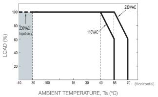
If 39.019 operates in cosntant current mode with the rated current, the maximum workable Ta is 55°C.
